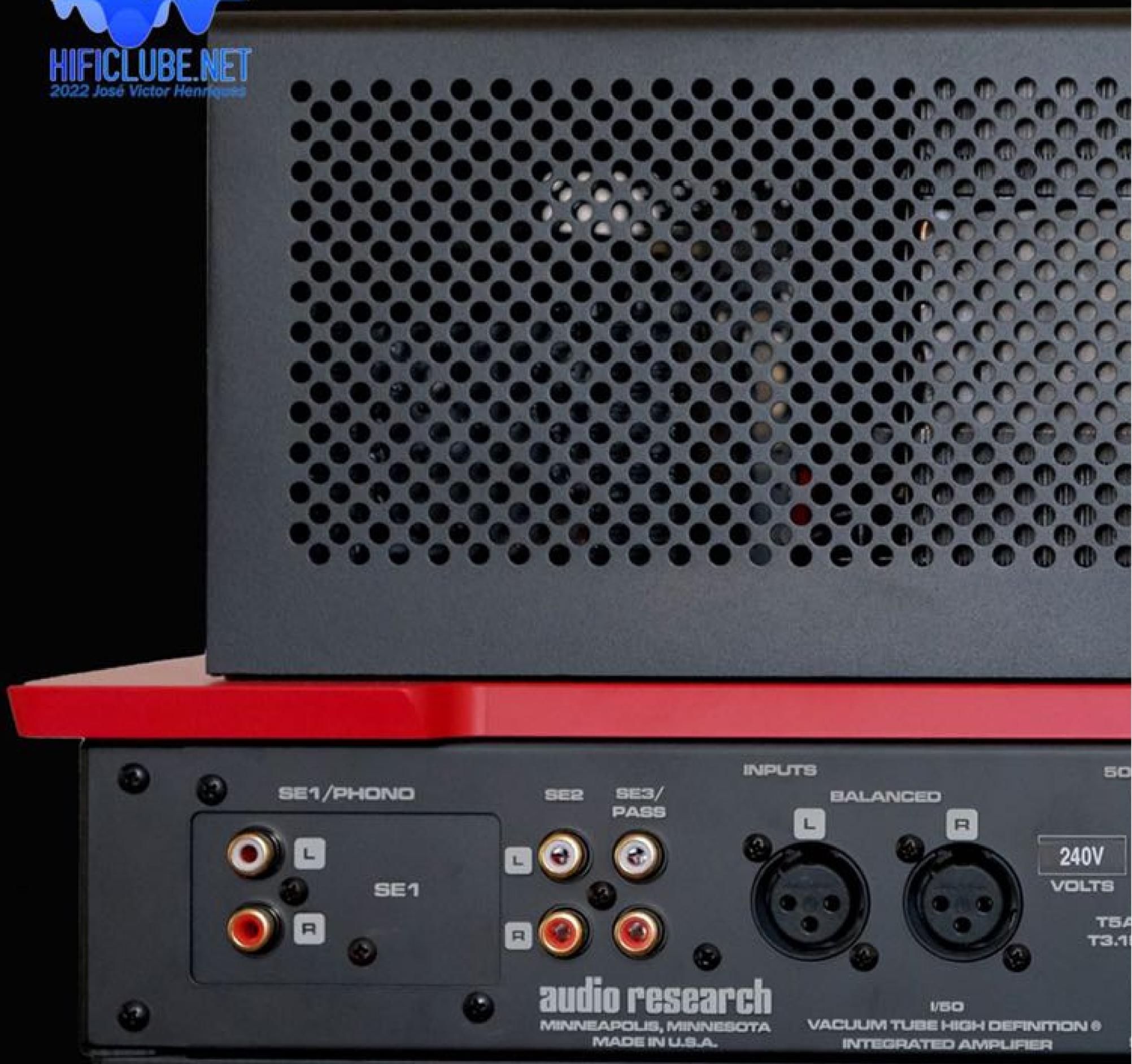
On the rear panel, we find three RCA inputs (No. 1 serves the Phono module when installed), No. 3 allows bypass when selected plus an XLR input. There is also a slot for the future DAC, which is already equipped with the appropriate inputs and outputs.
